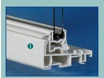
appearance ② while allowing maximum glass viewing .The engineered channels allow for dual layers of weather stripping to minimize air infiltration. Efficient "Warm Edge" insulated glass maximizes
